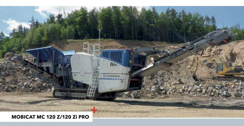
The MOBICAT MC 120 Z PRO, the first jaw crusher in the PRO line, is used for precrushing almost all types of natural stone. The jaw crusher is extremely robust and impresses with its low-maintenance operation. The machine therefore guarantees high production outputs.
