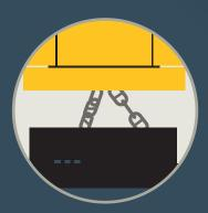
Built-in **generator with advanced control technology** provides faster material pick-up by a quick magnetization with impulse excitation and material release by automatic demagnetization with counter voltage and sequence pulsation.
