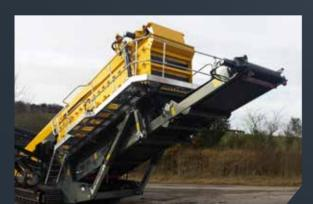
9.2 m<sup>3</sup> hopper, wide loading area Enables the use of wider loading buckets.
