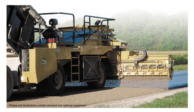
Front wheel drive ChipSpreader with standard spread hopper
