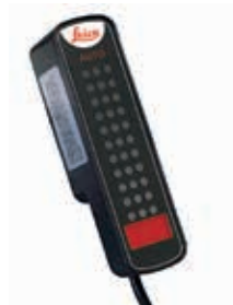
Arrow display indicating the bucket height
