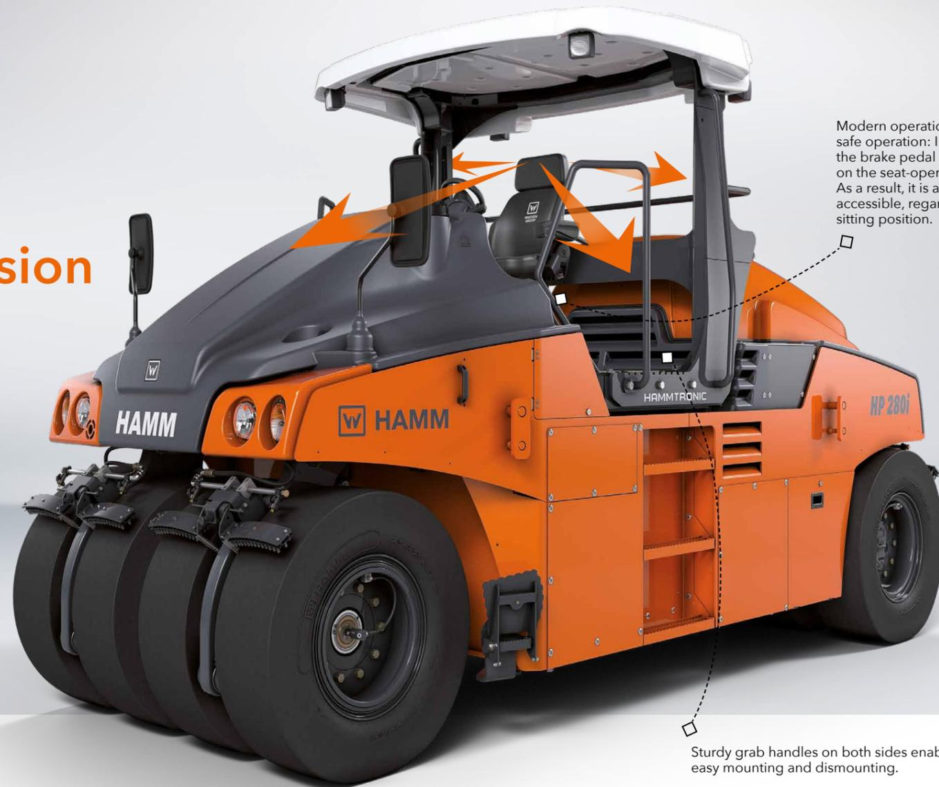
Modern operation – safe operation: In the HP, the brake pedal is located on the seat-operating unit. As a result, it is always easily accessible, regardless of the sitting position.
