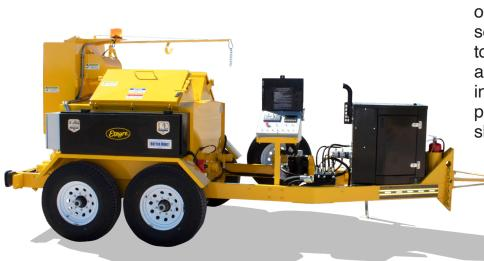
The Etnyre Crack Sealer is one of the most efficient crack sealing machines available today. The speed of the heating and circulation systems results in less crew idle time, higher production, and lower cost per shift on every crack sealing job.
