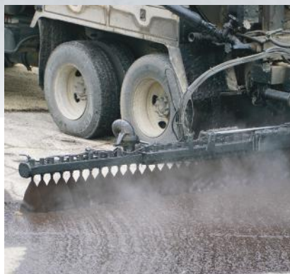
SOLID PIPE CIRCULATING SYSTEM
