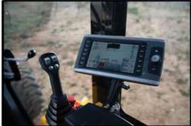
Single Joystick controls all moldboard, bucket, and scarifier functions. 7in color display shows engine parameters and control options.
