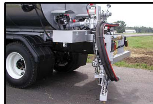
Precision Spray's exclusive center break-away system allows the bar to move if hit by an object.
