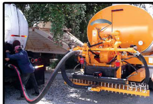
Load material using the Precision Spray 400 GPM asphalt pump. All pump functions pass through a single, self-cleaning strainer.
