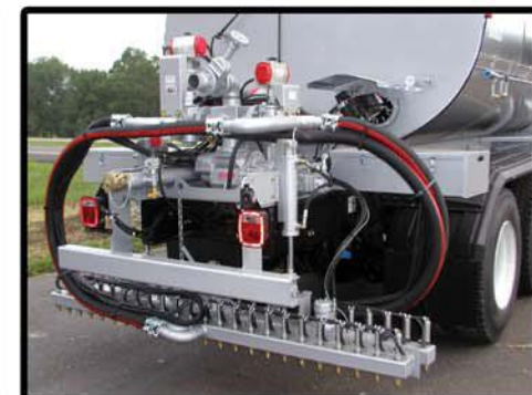
Easy access to the heated asphalt pump & control valves make the Precision Spray very service friendly.
