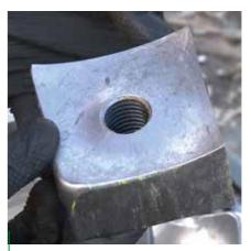
Bolt on cutting teeth Can be rotated to maximise wear part life
