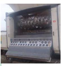
Medium speed shredder with aggressive cutting teeth
