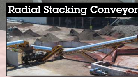
Radial Stacking Conveyor The radial stacking conveyor discharges a uniform end-product into independent bins for different colored products.
