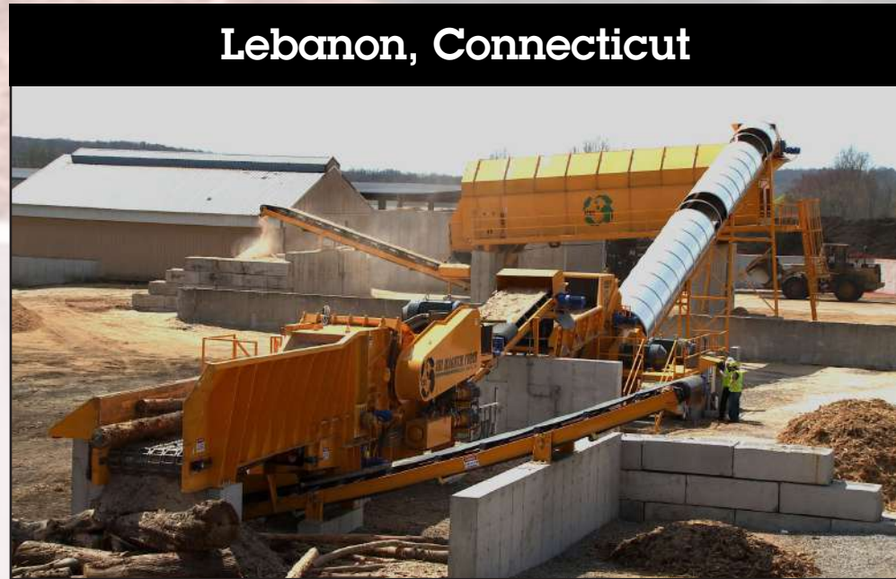
8400 Horizontal Grinder The primary horizontal grinder, the proven CBI 8400, has a 48" diameter x 60" wide downswing rotor. This solid steel drum rotor is powered by two 500 hp crusher duty electric motors. The custom infeed is extended for longer logs and features a screen on the feed hopper to remove dirt and rocks.
