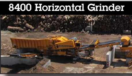
8400 Horizontal Grinder The primary horizontal grinder, the proven CBI 8400, has a 48" diameter x 60" wide downswing rotor. This solid steel drum rotor is powered by two 500 hp crusher duty electric motors. The custom infeed is extended for longer logs and features a screen on the feed hopper to remove dirt and rocks.
