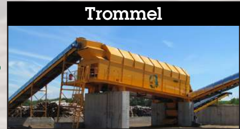
Trommel Any 1/4" minus fines are removed by the hexagon-shaped trommel which is totally enclosed for dust control.
