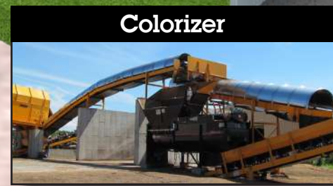
Colorizer The colorizer provides the operator with the ability to change colors and produce different colored end products at the push of a button.
