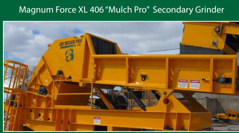
Magnum Force XL 406 "Mulch Pro" Secondary Grinder Providing high-volume mulch producers with a low cost per ton, the Mulch Pro is bigger, badder, and more versatile than anything made for this application. A split hog box design allows for easy maintenance access. The vertical feed configuration is ideal for secondary grinding. The rotor maintains high throughput of a precise product, bringing an enormous amount of material down to its final spec size. Owners can add watering or coloring systems to this design.
