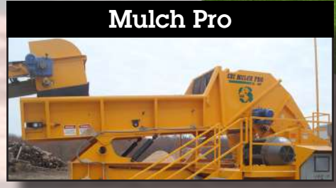
Mulch Pro Secondary grinding is accomplished by the CBI Mulch Pro XL 406. The vertical feed Mulch Pro has a 40" diameter by 60" wide steel drum rotor that grinds material to the final mulch spec.
