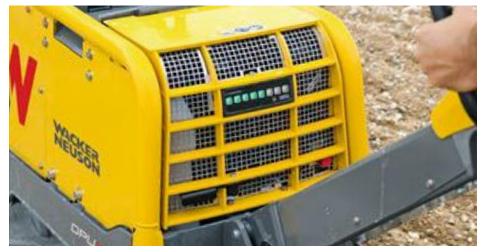
Compacec compaction control shows the operator when the best possible compaction has been achieved with this machine. This saves excess passes and time.
