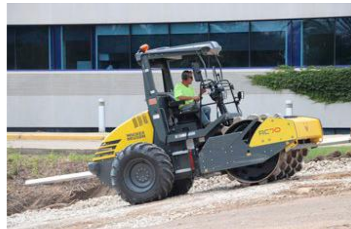
Traction control ensures that the wheels do not spin even on uneven terrain.
