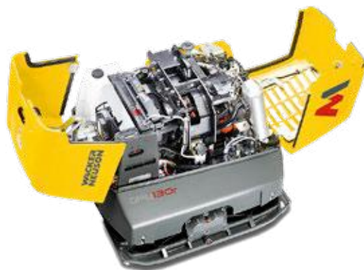
The best service access – simply fold open the cover.
