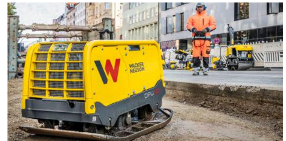
Intelligent proximity recognition sensor: The machine stops automatically when the minimum safety distance between the operator and the machine is less than 2 m.
