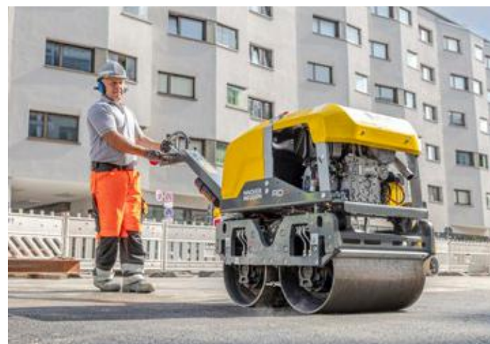
Long center pole facilitates steering and turning, especially in small areas.
